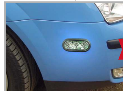
MicroLed Advance and Sputnik have fully interchangeable electrical connections for an easy installation.
