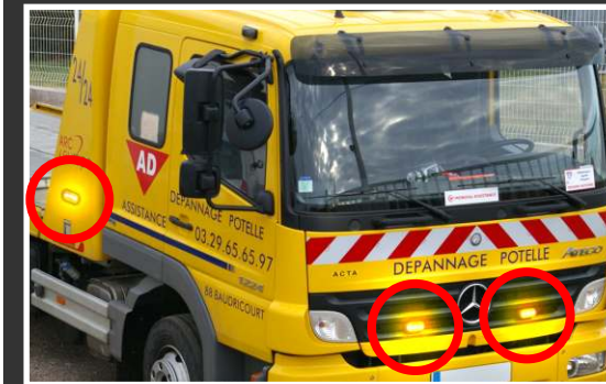
Special spread lens in blue, amber and red, following UN R65 European directive.
